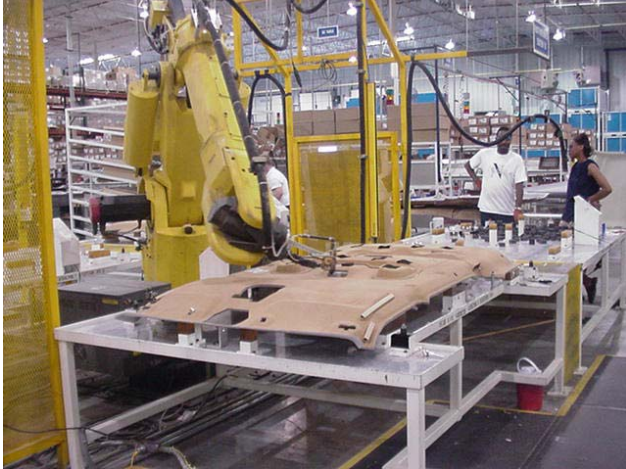
RFID tags attach to automobile parts coming down an assembly line. The tag is read by a transceiver, which communicates with I/O systems and PLCs controlling a robotic arm.
